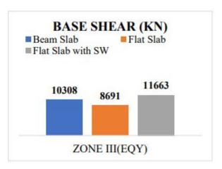
Figure 3: Base Shear(KN) in Zone III for EQX and EQY
