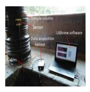
Figure 10: Experimental setup at the Amrutesvara temple
